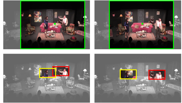
Figure 2. Video retargeting vs. editing: Video retargeting (top row) involves estimating the location of a cropping window (defined by the x -coordinate denoted by a green dot) that preserves focal scene content for rendering on a device with different aspect ratio. Video editing (bottom row) involves compositing several manually captured or virtually generated shots (two of the simulated shots are shown) to capture focal characters in vivid detail, and selecting at each instant the shot that most engagingly conveys the storyline. Selected shots are rendered at the same aspect ratio as the original video.
