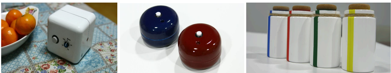
Figure 3. Three DDPs: music-playing light-sensing timer, wireless communicable objects, and jar-shaped sound recorders.
