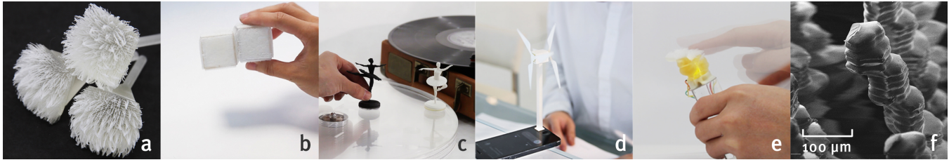
Figure 1. Printed Objects with Cillia. (a) Printed Flowers with fine surface details; (b) Mechanical adhesion surface; (c) Passively actuated dancing figures; (d) Ambient actuated object for notification; (e) Acoustic sensing of swiping gesture; (f) Scanning electron microscope (SEM) image of the printed hair structure.
