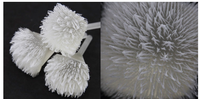
Figure 9. Successful printed hair arrays on curved surfaces.
