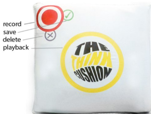
Figure 3. ThinkCushion interactive areas: record audio, save after recording, delete after recording, playback.
